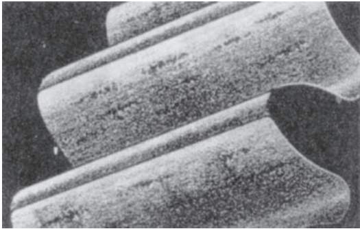
FIGURE 13.37. Pattern caused by corrosive attack on gear teeth.
